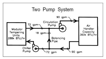
Figure 3: Diagram of a Typical 2-Pump System
