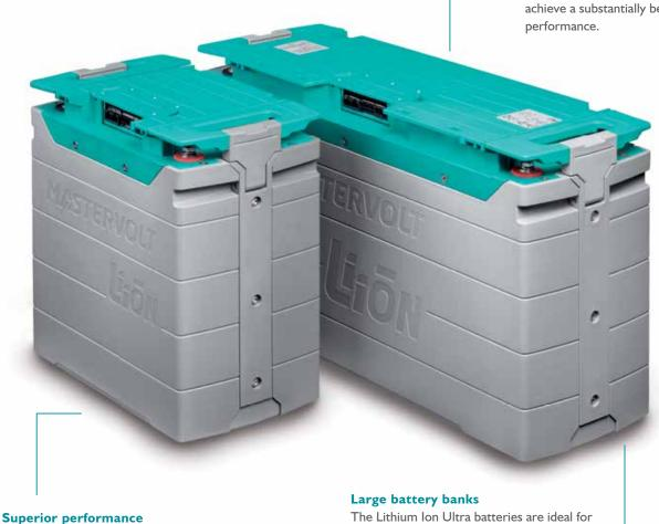
Mastervolt Lithium Ion batteries have a lifespan of over 2000 cycles at a depth of discharge (DOD) of 80%. This is three times longer than lead acid batteries thanks to features such as battery management, the almost complete absence of self discharge and the minimal build-up of the infamous 'memory effect'.
