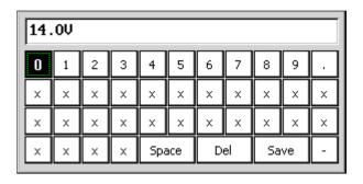
When prompted to change a numerical value for High/Low Limits, Current/Voltage settings, you will see a Numerical keyboard. It is used exactly the same as the Text/Numeric Keyboard. Note, the unit of measure (V,A etc) does not need to be entered. It is set by default.
