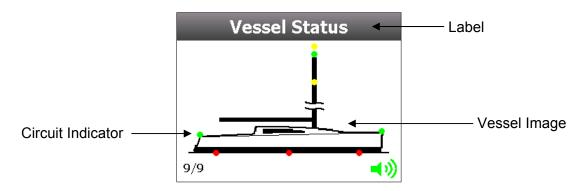
The Mimic page will give the user a view of all systems in operation circuits on a selectable boat image. The 5 default boat images can be chosen from the following:
