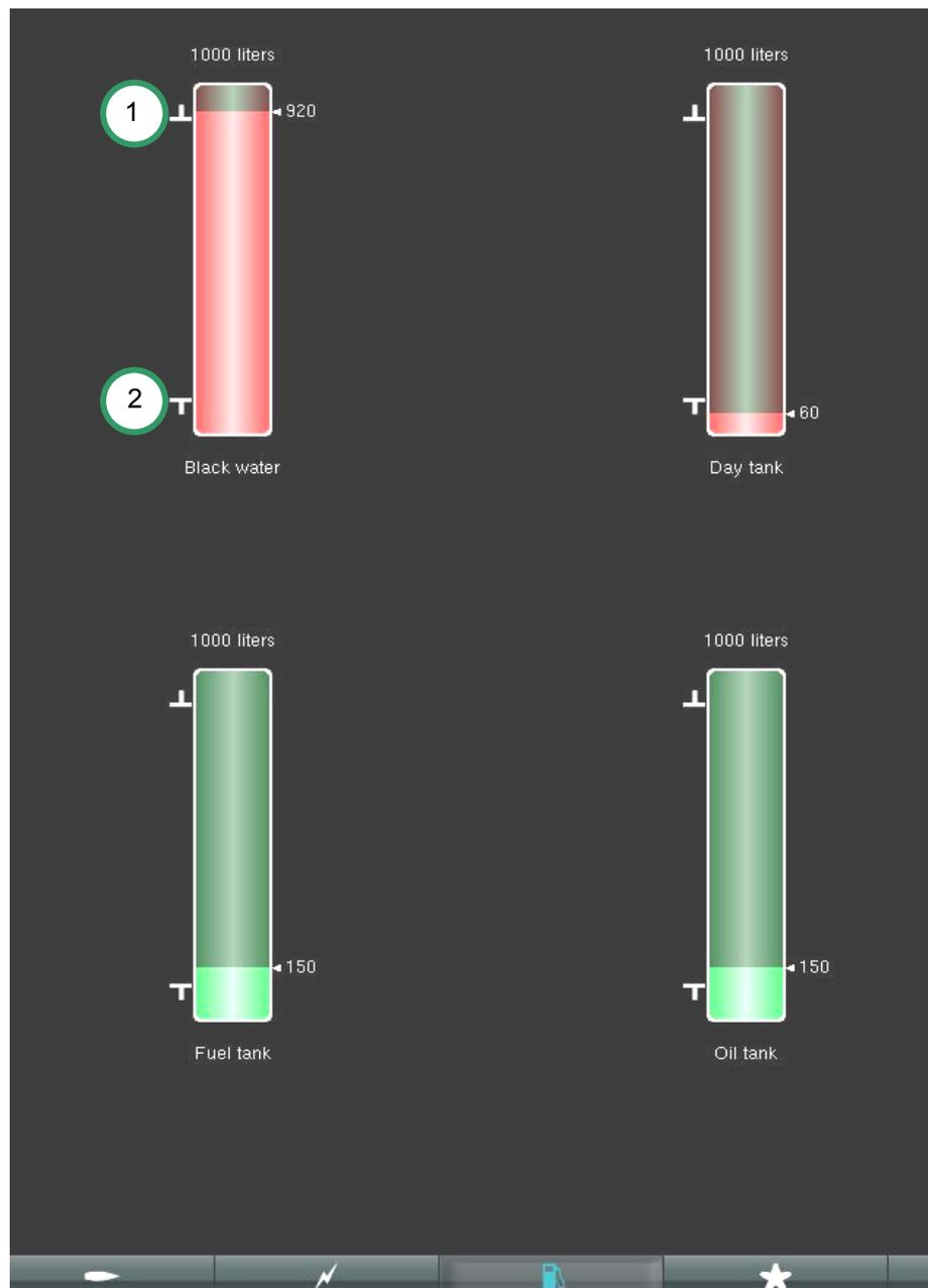
Figure 26: Tank level screen
